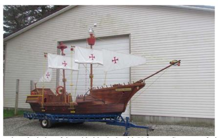
2. Insert both Masts into the holes of the mid-ship deck with Velcro on Crosstrees facing the bow. The bell on the Mainmast faces to the rear.
