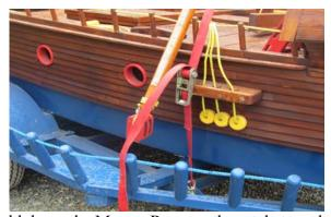
1. Untie both ratchets that hold down the Masts. Remove the ratchets and store in the storage space in mid-ship. See Picture above #6 that shows storage space.
