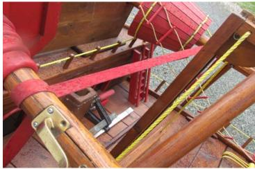
9. Tie both Masts down with the ratchet tie downs. Place the hook of one ratchet set in the rear eyelet on the trailer frame at the back, loop over and around one mast, cross over to the other mast and loop over and then down to the other side eyelet on trailer frame. Ratchet until tight. DO NOT over tighten as the mast may break.
